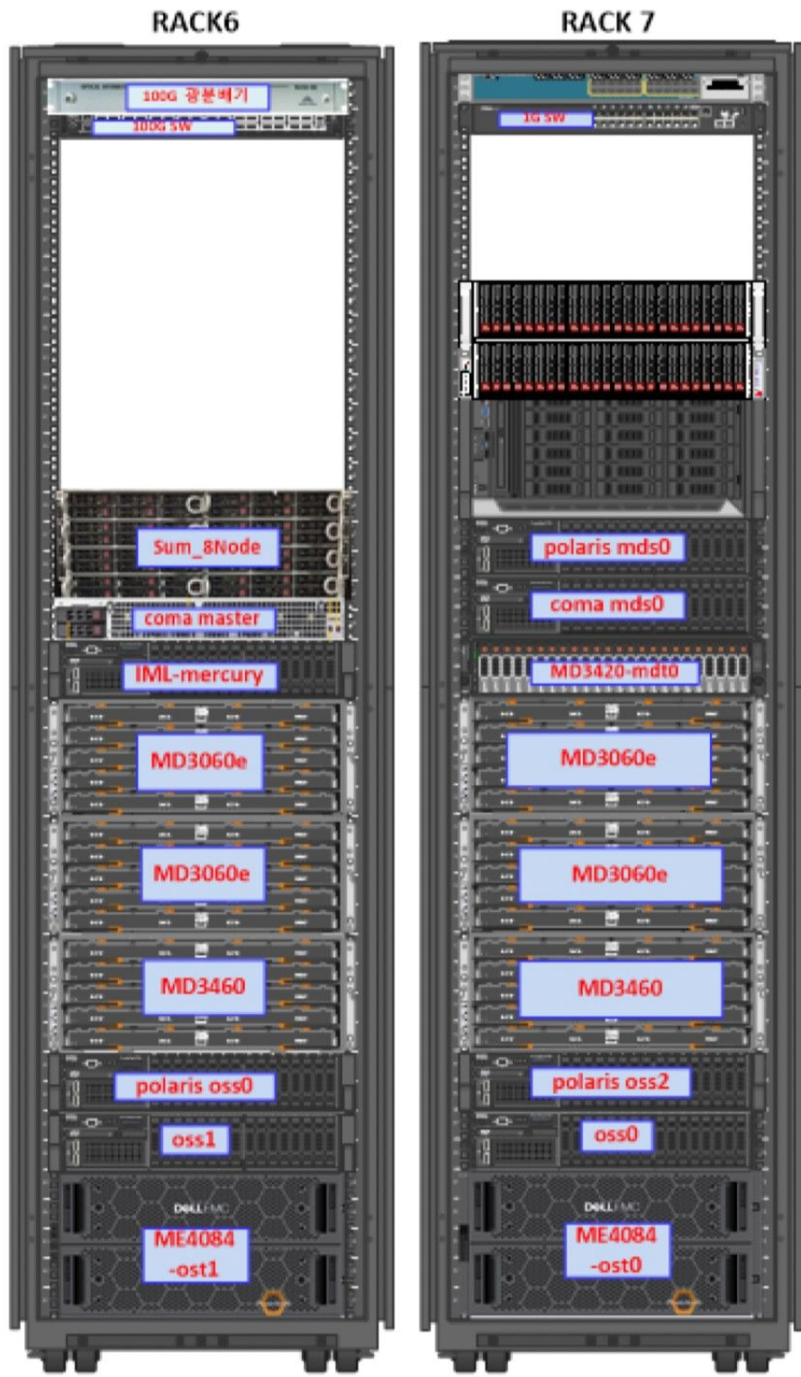
Figure 19: A computing cluster and Lustre file system dedicated for the software correlation of the KVN.
