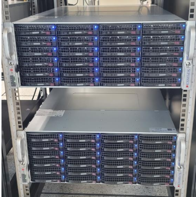
Figure 17: Front view of the two Flexbuff units at KPC. 24 disks are mounted for one Flexbuff.
